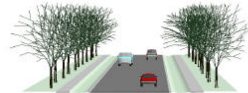
Figure 7.4.c A 66 foot Right-of- Way with 6 foot swales, street trees, curb, sidewalks and 24 feet of pavement. Street trees shown in swale or outside of sidewalk.
