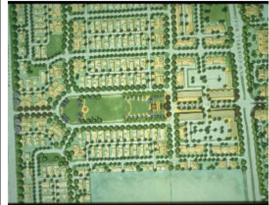
Above, a variety of street widths appropriate to the varying level of travel and parking needs in a community.
